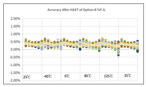
Figure 21. Option B accuracy after HAST
