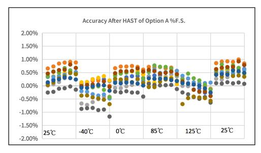
Figure 20. Option A accuracy after HAST
