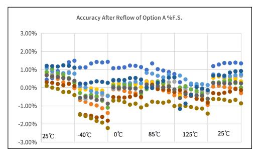
Figure 14. Option A initial accuracy after reflow
