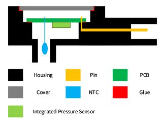
Figure 3. Cross-section of a TMAP Module
