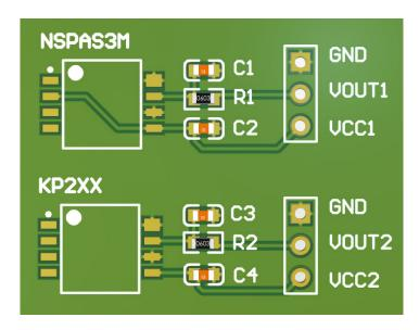
Figure 5. Pin to pin compatible demonstration
