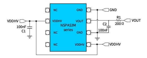
Figure 6. Application circuit of NSPAS3M
