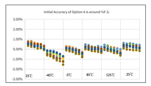
Figure 11. Option A initial accuracy
