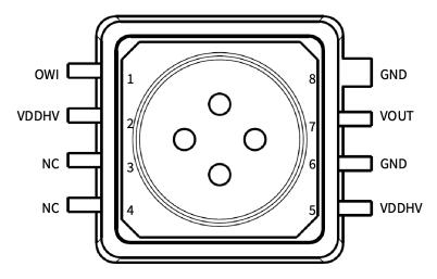
Figure 4. Pin definition of NSPAS3M series
