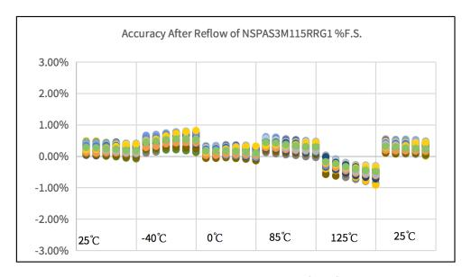
Figure 13. NSPAS3M115RRG1 accuracy after reflow
