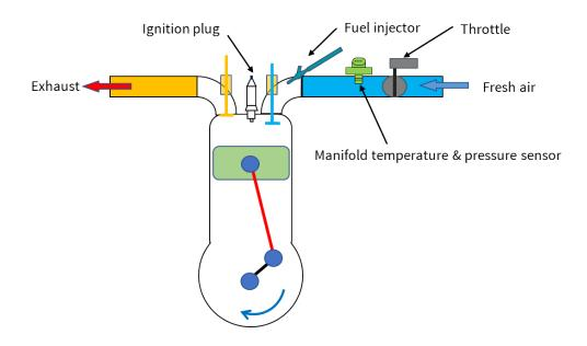
Figure 1. Electronic fuel injection system for automotive and motorcycle
