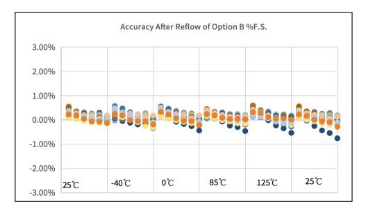
Figure 15. Option B accuracy after reflow
