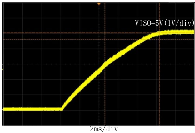
Figure 5.2 5V→5V Soft start at full load
