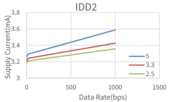
Figure 5.2 NSI8266 VDD2 Supply Current vs Data Rate
