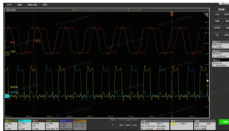
Figure 8.4 NSI8366 driving signal with interlock triggered
