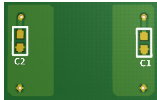
Figure 9.3 Recommended PCB Layout — Bottom Layer
