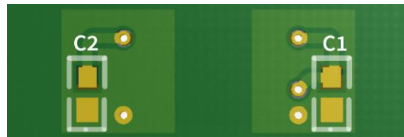
Figure 9.3 Recommended PCB Layout — Bottom Layer
