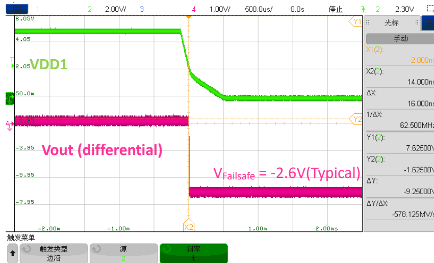
Figure 8.4 Typical Failsafe output when VDD1 undervoltage
