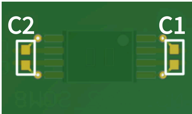
Figure 9.3 Recommended PCB Layout — Bottom Layer
