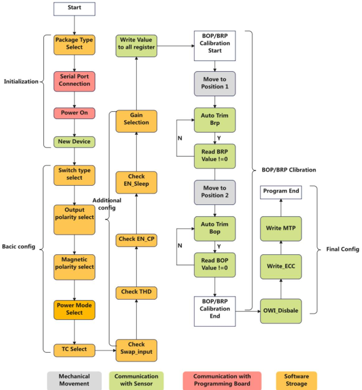
Figure 3.12 Full Configuration Flow
