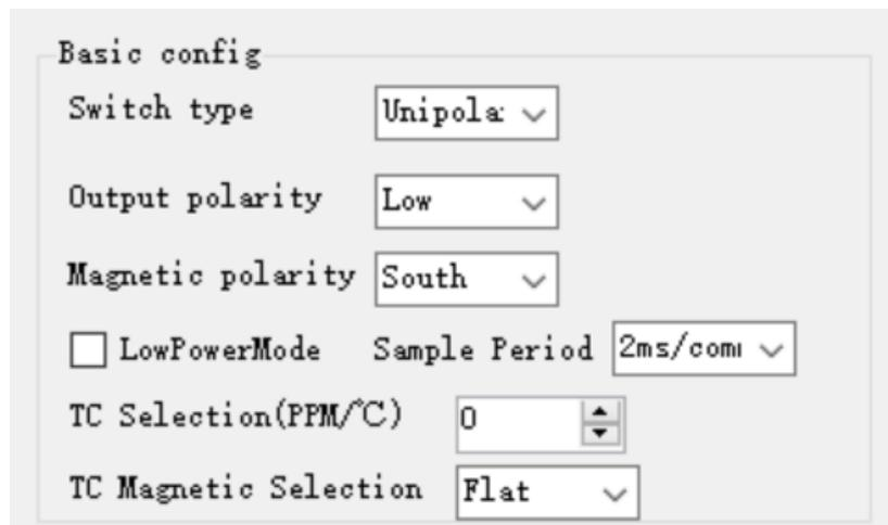
Figure 3.5 Example of Unipolar South Standard Polarity
