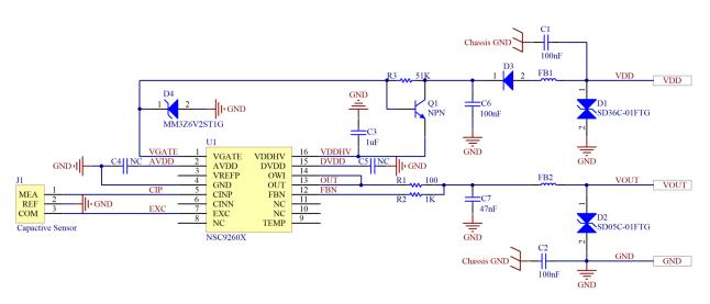
Figure 3.3 Schematic of Analog Voltage Output with High Voltage Input (BJT)
