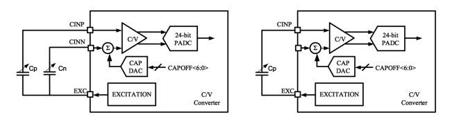
Figure 2.1 Capacitive Sensor Connection Diagram
