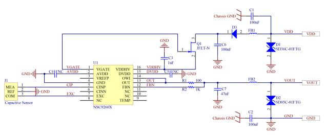
Figure 3.2 Schematic of Analog Voltage Output with High Voltage Input
