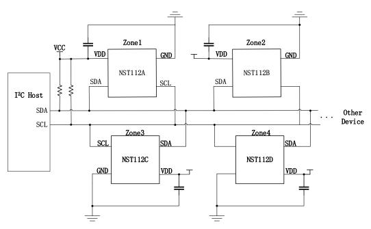
Figure 6. 2 Application Diagram
