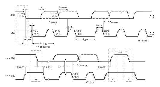
Figure 4.1 I<sup>2</sup>C Timing Diagram
