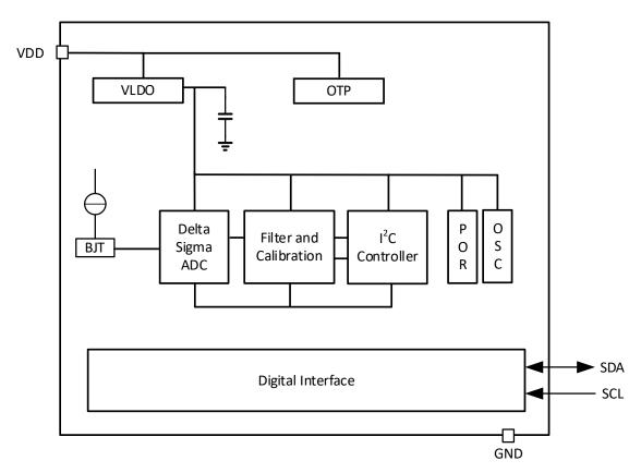
Figure 5.1 NST112 Functional Block Diagram
