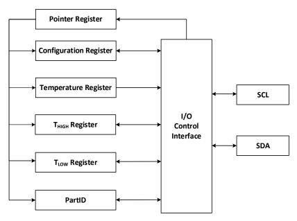
Figure 5.4. On-chip Register Structure
